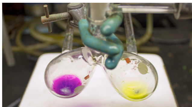
Figure 1. Apparatus for gas phase H 2 transfer from a solution of 1b,d (yellow solution in right bulb) to a solution of 3 (purple solution in left bulb) through an evacuated headspace. 16
